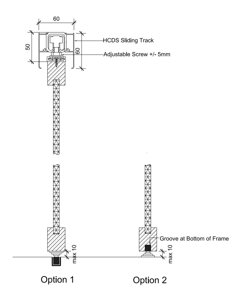
Typical Detail | Sliding Screen System | Scale 1:2 @A3
